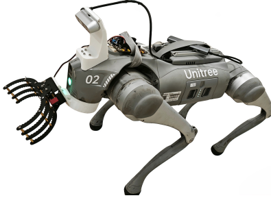
Figure 4: Hardware Setup. The overhead D435i camera is mounted at a fixed pitch alongside an ultra-low-cost servo-driven two-finger gripper using brackets [15].
